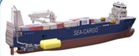
LNG powered vessel design (source: DNV)
